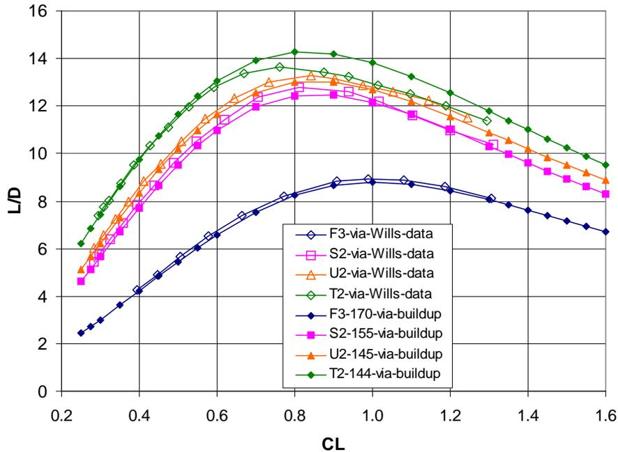
**Figure 15. Comparison of L/D estimates with manufacturer's data**
