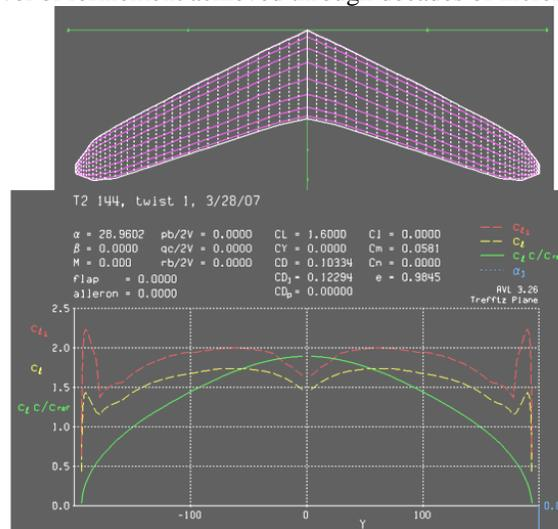
**Figure 12. T2 Induced drag estimate using AVL.**
