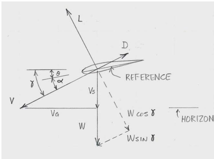
**Figure 10. The geometry of gliding flight**
