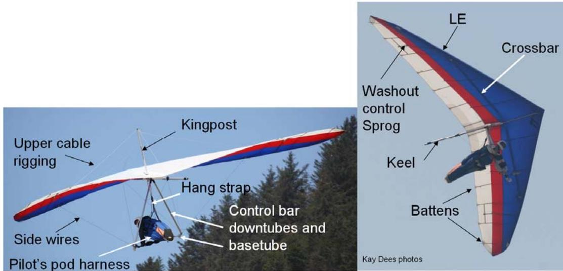
**Figure 3. Flex-wing hang glider parts**
