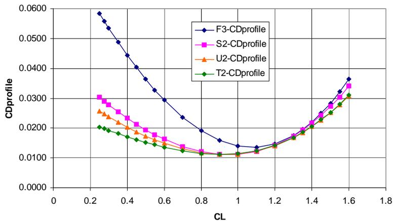
**Figure 14. Adjusted profile drag estimates**
